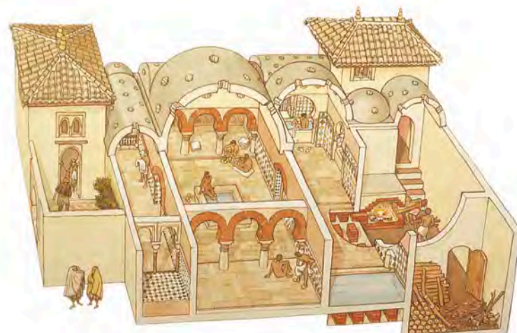
Below, typical Moorish baths, al-hammam in Arabic, origin of the name Alhama. They consist of a courtyard, hall, cold room, warm room with pool and the hot room, where the steam and hot water is produced by a boiler.
